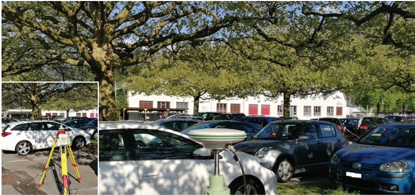
FIGURE 7 Test setup under canopy in Heerbrugg (rover: GS10, antenna: AS10).
