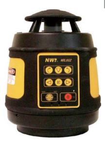
Laser Beam: Horizontal & Zenith Wave Length: 635 nm Operating Range: 2,000 ft with Detector Leveling Accuracy: 1/16 in @ 100 ft horizontal 1/8 in @ 100 ft vertical Self Leveling Range: +/- 5° Tripod Adaptor: 5 / 8 x 11 thread Includes: Remote Control, Bracket, Grid Target, Glasses, Batteries & Charger, Carrying Case & Manual
