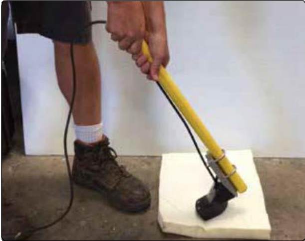
7.A: Place transducer on protective pad.
