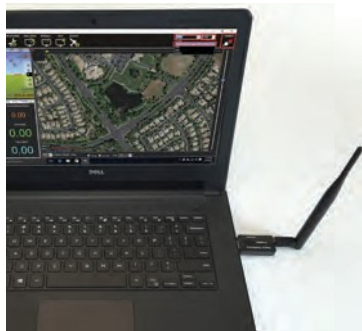
Figure 5: Attach USB Radio Telemetry to the Mission Planner Laptop.
