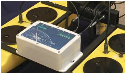
Figure 1—Attach AutoNav control module to the Pontoon frame.
